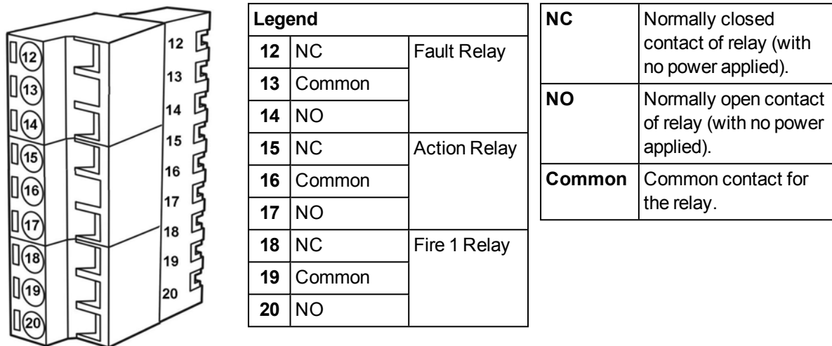
Figure 2-12: Terminal block display, relays
